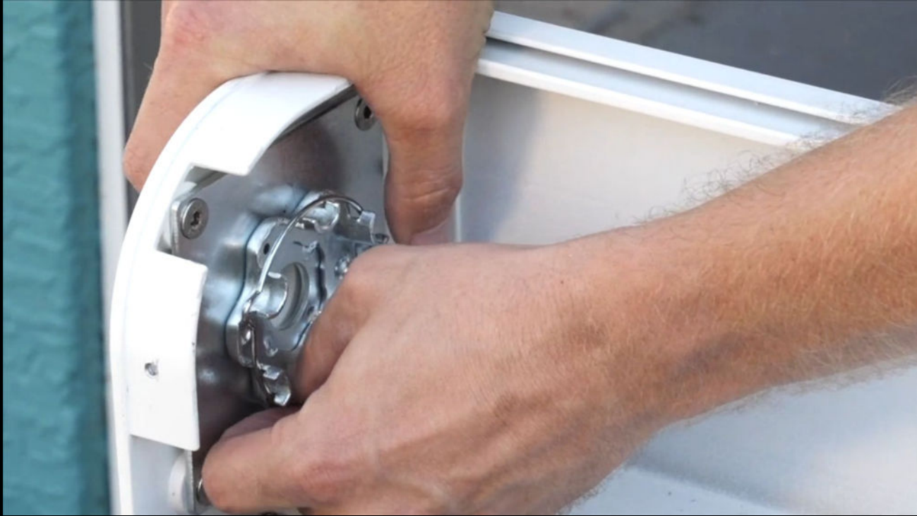
Re-attach motor clip to motorside housing
